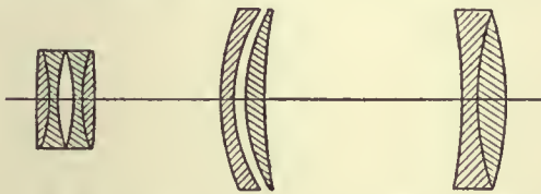
FIG. 57.—T. R. Dallmeyer's Compound Telephotographic Lens.
